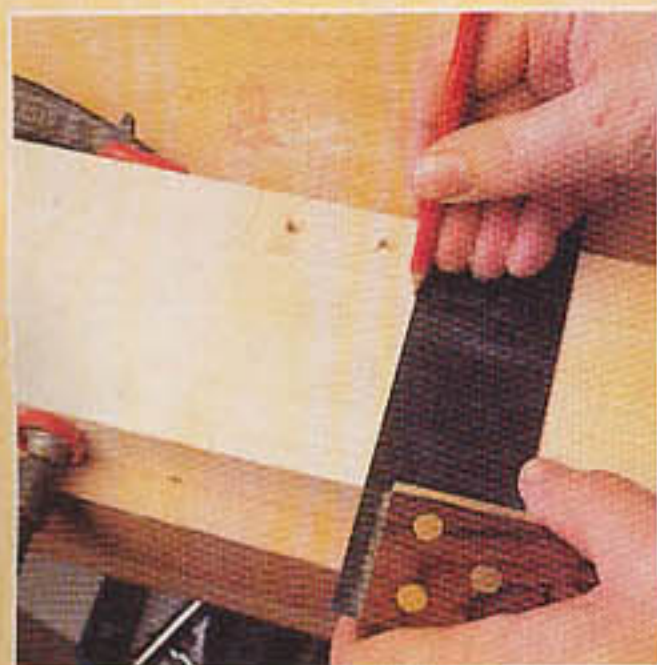
9 Mark out one upright as a pattern piece and transfer the measurements from this to a batch cramped together
