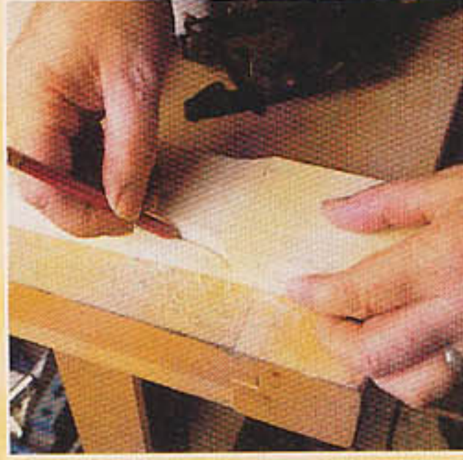
14 Draw out and cut a decorative cutaway on either side of a seat back slat and use this as a pattern to mark the rest
