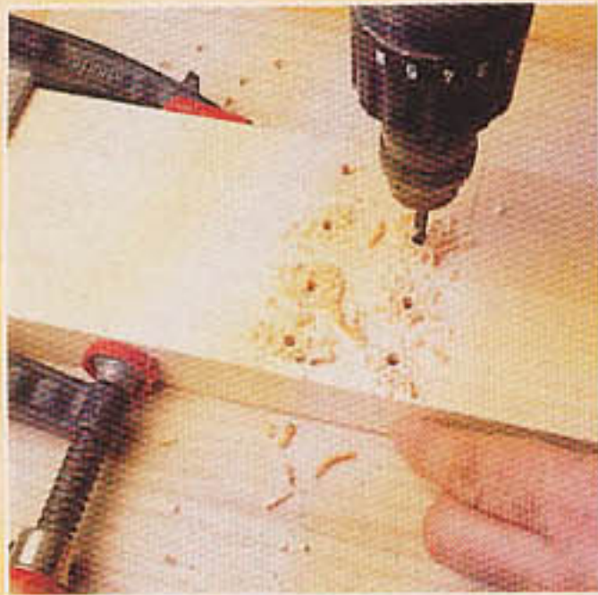
10 Drill a clearance hole and countersink for each fixing screw to ensure that it will not split the timber especially at the ends
