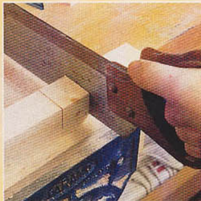
3 Hold the rail firmly in a vice or on a bench hook while you cut the joint cheeks. Use a tenon saw and saw just to the waste side of the line down to the gauged shoulder
