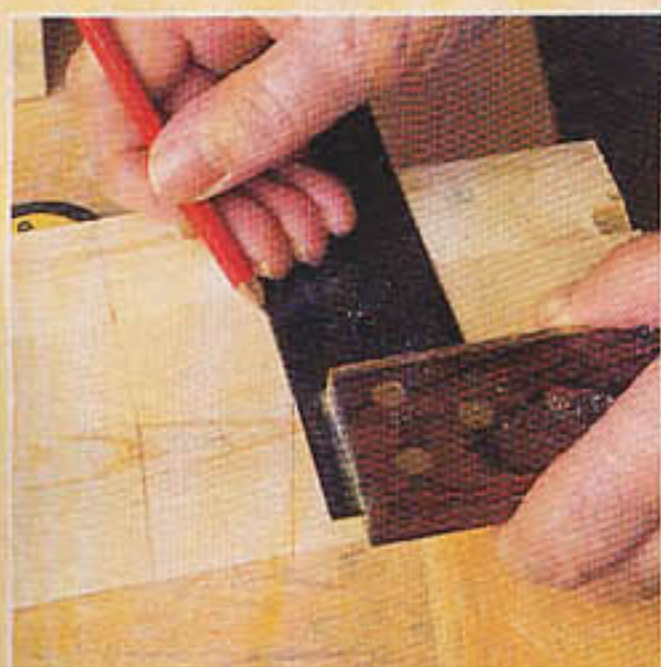
1 Mark out identical rails in sets. Cramp them together and square the joint markings across the top faces, then separate the timbers and square the lines around each piece
